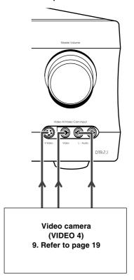
The VIDEO 4 INPUT jack is equipped with a protective cap. When using this jack, remove the protective cap and keep it safely. When not using this jack, replace the protective cap.
